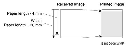
**NOTE:** The upper limit (page length + 20 mm) is adjustable between 0 and 155 mm. Refer to Printer Switch 04, bits 0 to 4 for more details.
