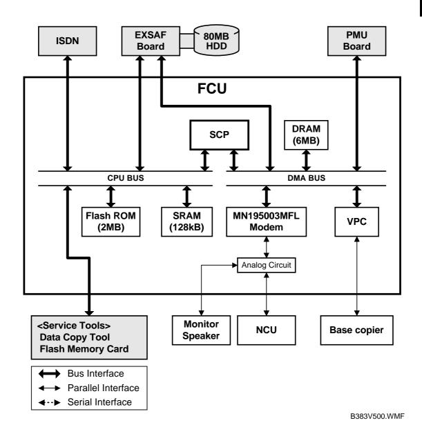
The basic fax unit consists of two PCBs: an FCU and an NCU.
