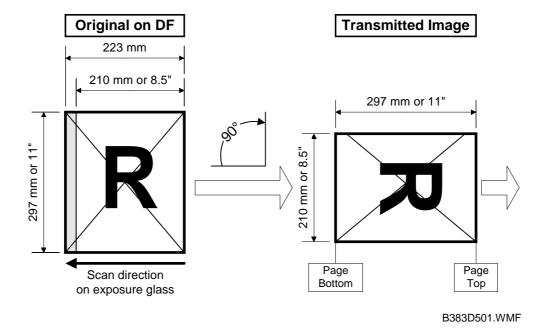
When this feature is enabled, in the above example, the gray part of the original is not scanned. However this allows the machine to rotate the image before transmission in order to avoid unintentional reduction.
