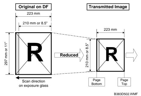
In the above example, this feature is disabled. An unintentional reduction may occur if the receiving machine cannot print on paper with a width of 297mm. However, with length-correction disabled, the machine sends the entire image.
